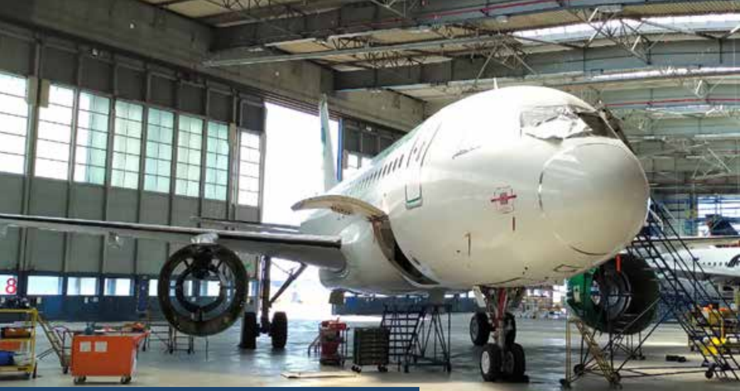
An A319 waiting for its two CFM56 Engines to be reinstalled after repair
